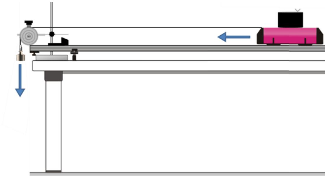
2. Place the cart at the end of the rail and attach a 50g weight to the clip.
